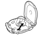
2 Insert the rechargeable battery so that the word "SONY" is facing the same direction as illustrated on the lid
