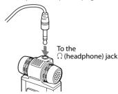
\*3 These buttons and the jack have a tactile dot. Use it as a reference point for operations, or to identify each terminal.
