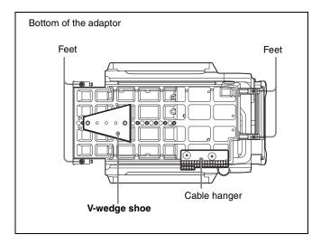
When attaching the V-wedge shoe, taking the total weight of the adaptor, camera, studio lens and viewfinder, and the size of the pan and tilt head of the tripod into consideration, choose a position such that the unit will be mounted stably on the tripod.
