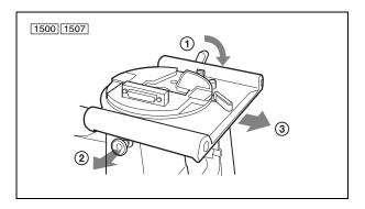
**2** Push the rear panel lock release lever on the left panel down to open the rear panel.
