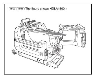
(5) Press the camera lock lever on the front panel fully downward to secure the camera in place.
