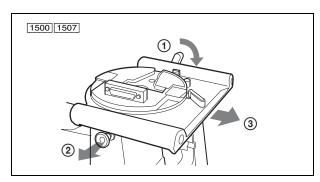
**3** Push the rear panel lock release lever on the left panel down to open the rear panel.
