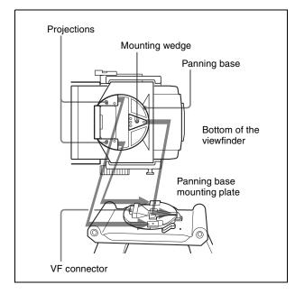
**2** Push the viewfinder by the handle so that the panning base is held securely by the panning base mounting plate.
