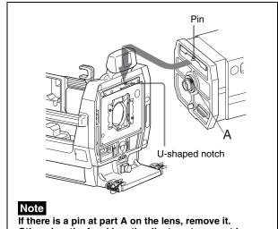
If there is a pin at part A on the lens, remove it. Otherwise, the focal length adjustment may not be made. If the pin cannot be removed, consult your Sony representative. **3** Push the rear face of the lens onto the front face of the lens adaptor then turn the lens lock holding knob clockwise.
