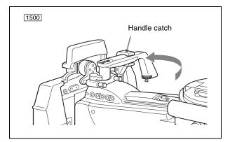
**3** While pulling the release knob ① on the left side to release the viewfinder table, slide the table as ② to an appropriate position. Then push the lock lever ③ toward the front to lock the viewfinder table in place.
