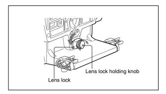
**2** Insert the pin on the rear of the lens in the U-shaped notch on the front of the lens adaptor.
