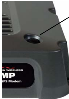
Figure 4-2: The MP modem reset button.
