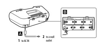
Connect the AC power cord A or insert six R20 (size D) batteries (not supplied) into the battery compartment B.
