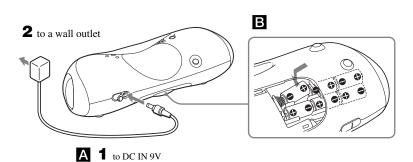
Connect the AC power adaptor A or insert six size C (R14) batteries (not supplied) into the
