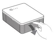
2 Insert the print cartridge to the back in the arrow direction until it clicks into place.
