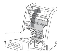
After removing the labels attached at both sides of the paper roll, place the paper roll in the paper holder.
