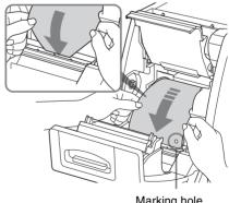
Be sure to remove all of the seals attached to the paper roll. A seal remaining inside the printer may cause problems.
