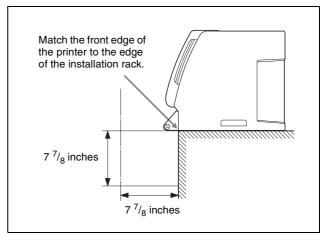
If there is not enough space (as shown in the illustration above), ejected printed sheets may pile up and clog at the Paper Output Slot and trouble may occur.
