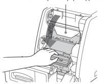
If the tip of the paper protrudes from the platen roller, be sure to insert the tip of the paper under the rollers.
