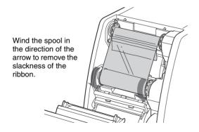
The ribbon is ready to be used. Depending on the position of the break in the tape, the ribbon for one sheet of printed paper may be lost.
