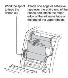
2 Turn the lower blue spool in the direction of the arrow to remove the slackness of the ribbon.
