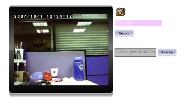
Click **Record** to activate this function. Press **Record** button to start recording. The video file is saved as ASF format into your local PC. While you want to stop it, press **Stop** to stop recording. Select **Browser**, the pop-up window to select the save path and file name prefix, select **OK** to continue.
