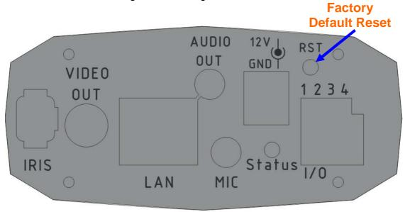
**Note:** Restoring the factory default setting will lose the all previous settings included IP address forever. User needs to run the IPWizard program to search the device and configure it to let the device work properly again.
