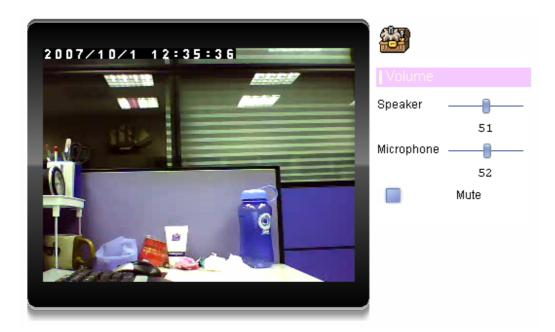
Click **Volume** to activate this function. There are two control bars for speaker and microphone volume respectively. Scroll these control bars to adjust the audio attribute. Check the volume mute will mute the speaker output.
