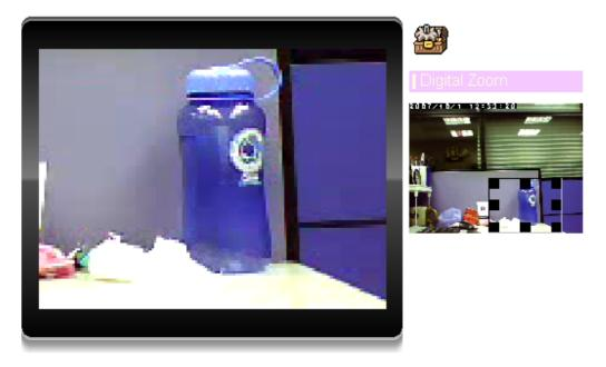
Click **Digital Zoom** to active this function as above. User can drag or scale the box over the video to adjust zoom ratio and position.
