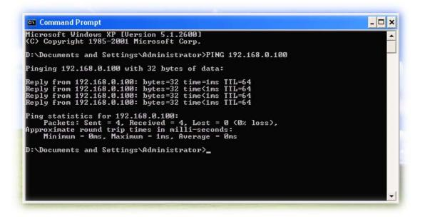
If you want to detect any other devices conflicts with the IP address of Network Camera, also can utilize the PING command but you must disconnect the device from the network first.
