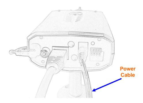
Once you have installed the camera well and powered it on, the power LED will turn on. It means the system is booting up successfully. Furthermore, if you have a proper network connection, and access to the camera, the LED will flash green under wired mode.
