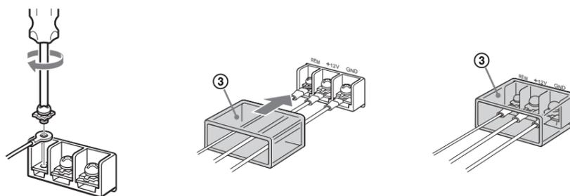
Pass the leads through the cap, connect the leads, then cover the terminals with the cap.
