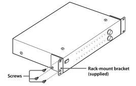
4 Mount the Component Video Switcher into the rack as shown below.
