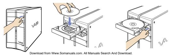
Mhen the computer is in **Standby** or **Hibernate** mode, you cannot insert or remove a disc.
