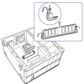
4 To insert a new memory module, remove it from its anti-static package, handling it only by the edges.
