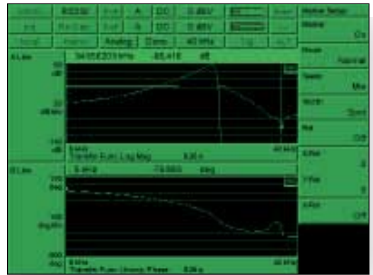
Swept-sine Bode plot of lowpass filter response. Top display shows magnitude with an expanded view of the passband response, while bottom display shows the phase response.
