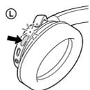
Press and hold the POWER button for about 2 seconds while this unit is turned off.
