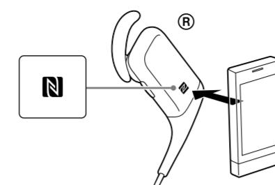
By touching the unit with a smartphone, the unit is turned on automatically and proceeds to pair and connect via BLUETOOTH.
