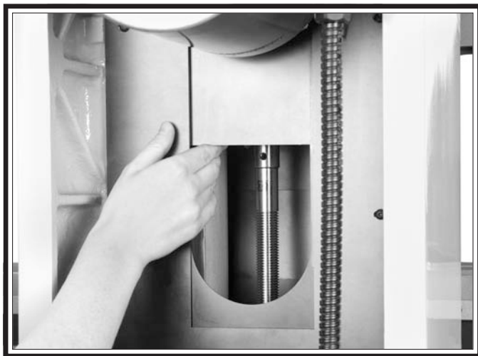
Figure 46. Upper leadscrew inspection.
