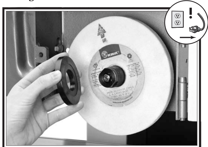
Figure 25. Wheel ready for removal.
