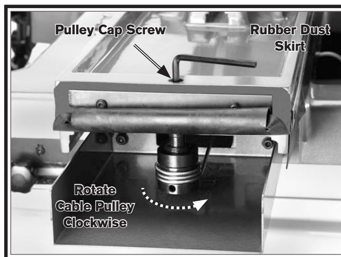
Figure 49. Adjusting cable pulley.
