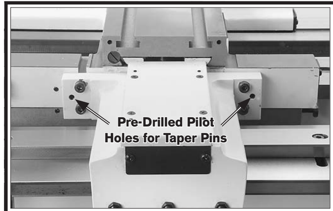
Figure 23. Taper pin pilot holes.
