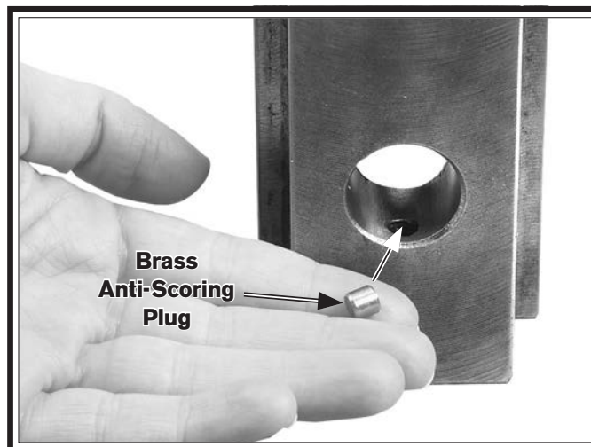
Figure 9. Slide block brass anti-scoring plug.
