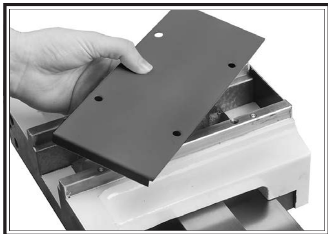
Figure 7. Attachment body top cover removed.
