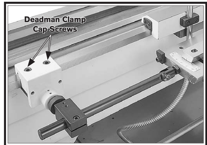
Figure 27. Deadman clamp cap screws.
