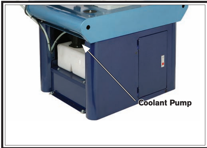
Figure 54. Coolant pump motor location.
