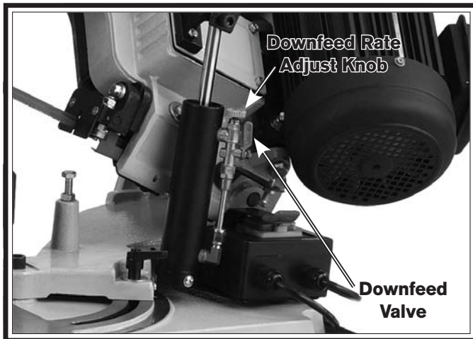
Figure 37. Downfeed rate controls.
