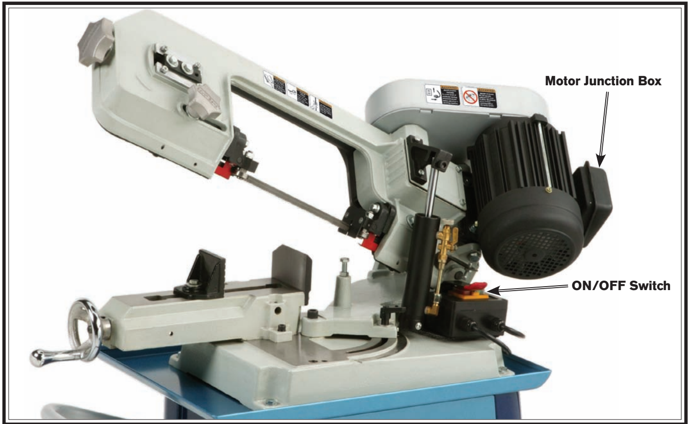
Figure 55. Wiring component locations.
