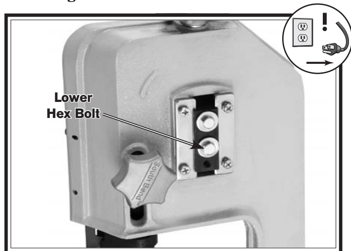
Figure 45. Blade tracking adjustments.
