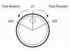
Inside the shuttle ring is the jog disk, shown in the illustration below, it can turn completely in either direction. Once you freeze the video, you can use the jog disk to go to single-step play back. Clockwise rotation causes forward one-step playback; and counterclockwise rotation causes backward one-step playback.
