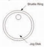
It is a combination of a shuttle ring with an embedded jog disk, which is used to provide wide latitude in playback control. Note that the jog/shuttle knob is active only when the DVR unit is in Playback mode.
