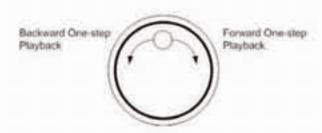
While playing back video, you can use the shuttle ring to select different speeds of forward and backward playing. Rotating the shuttle ring counterclockwise causes the unit to playback in fast forward/ backward playing speed. According to the angle you rotate the shuttle ring, you can choose the playing speed from 1x, 2x, 4x, 8x, 16x, and 32x, in both forward and reverse directions, shown in the figure below:
