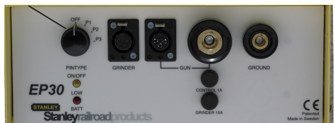
Figure 3. Pin Type Control Switch
