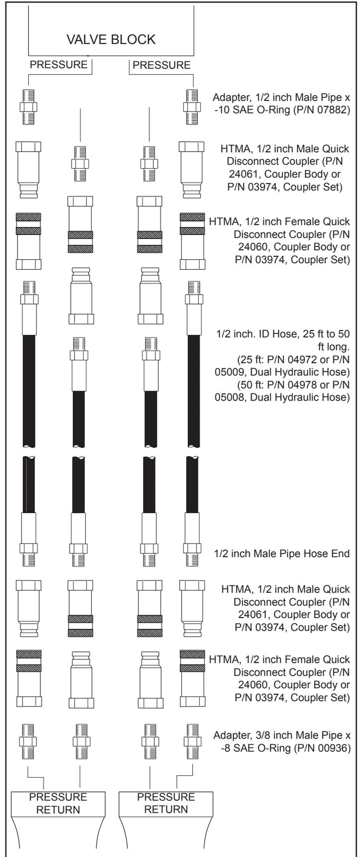
Figure 2. Hydraulic Connections
