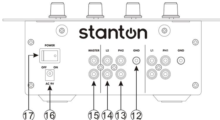
12. Ground - Grounding post for turntable connection. Always use this connection when using standard turntables with ground cable. (Some turntables like the STR8-80 /100 do not require grounding wire)
