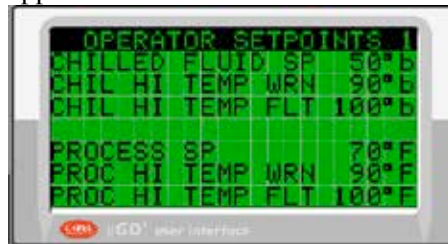
Figure 15: Operator Setpoints Screen
