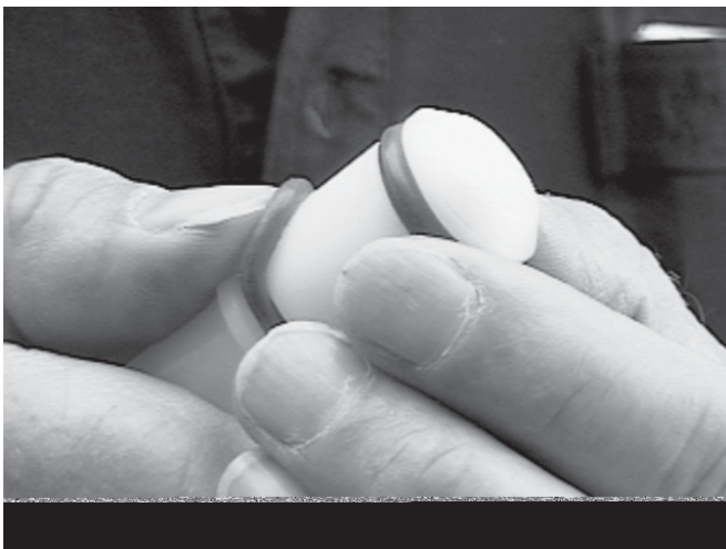
Figure 23. Removing "O" Ring
