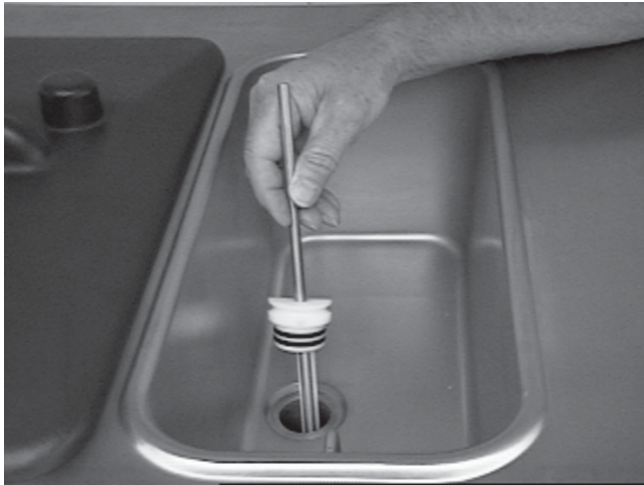
Figure 16. Removing Mix Inlet Regulator
