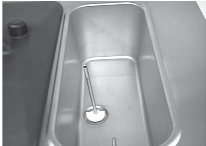
Figure 26. Install Mix Inlet Regulators
