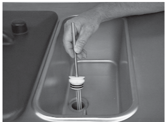
Figure 16. Removing Mix Inlet Regulator
