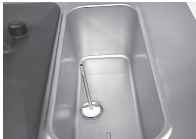
Figure 27. Install Mix Inlet Regulators
