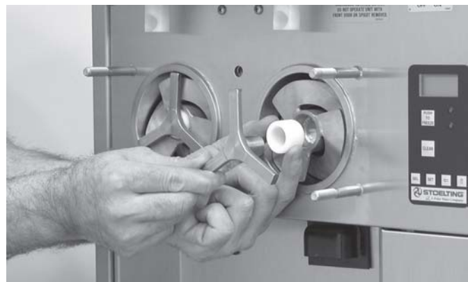
Figure 23. Removing Auger Supports
