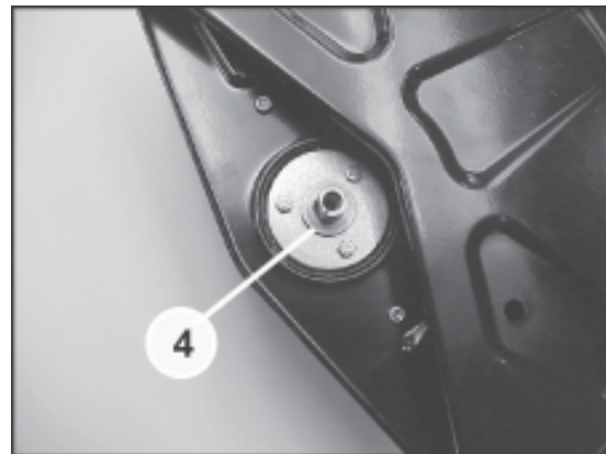
Figure 7. Selecting the Proper Blade Arbor
