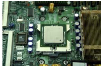
Socket lever in the locking Position
