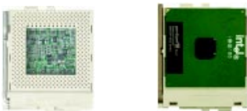
Figure 5-3A. FCPGA Socket: Empty and with Processor Installed
