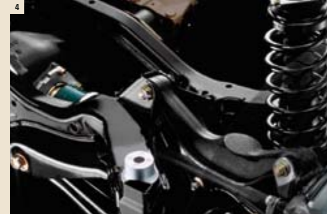
4 A sophisticated, reengineered multi-link rear suspension features newly revised geometry. It's designed to offer greater resistance to roll when cornering, and helps resist squatting during hard acceleration.
