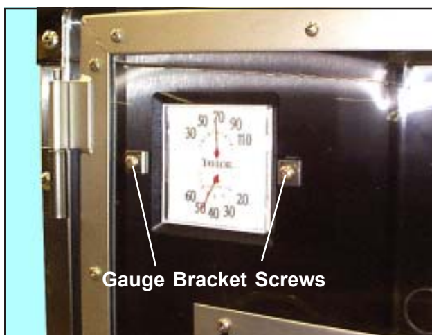
Figure 22. Removing the Old-style Gauge Assembly
