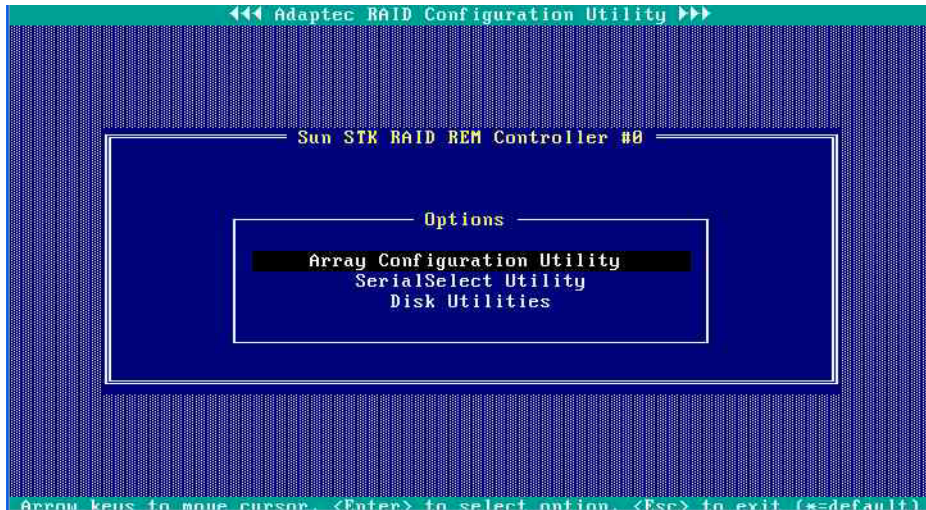
FIGURE B-1 Adaptec RAID Controller Utility (ARCU) Initial View
