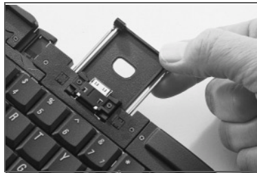
Retracting the docking mechanism
