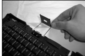
Extending the docking mechanism and PDA foot
