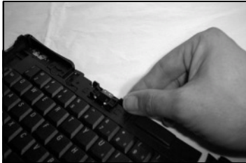
Extending the docking mechanism and PDA foot
