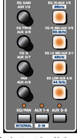
Sonar can come with up to three types of EQ, depending on the version you have. The FW-1802 can be set to control any of the three:
