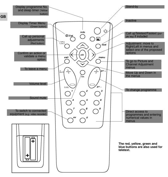
**Batteries:** Remove the lid at the back of the remote control and insert two 1.5 V. LR06 batteries.
