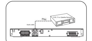
To listen the sound from your VCR, TV or Satellite Receiver through the speakers of this unit, only connect the Left / Right audio output of these equipments to the
