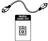
Optical socket and cable for digital audio signal.
