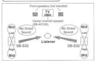
The SB-S32 reproduces low frequency signals from the front and mid-to high frequency signals from the rear. With Technics specially developed mode, the dipole sound field shown in the below figure is created around mid range signals. This means the listener can enjoy natural surround effect without being bombarded by direct sound.
