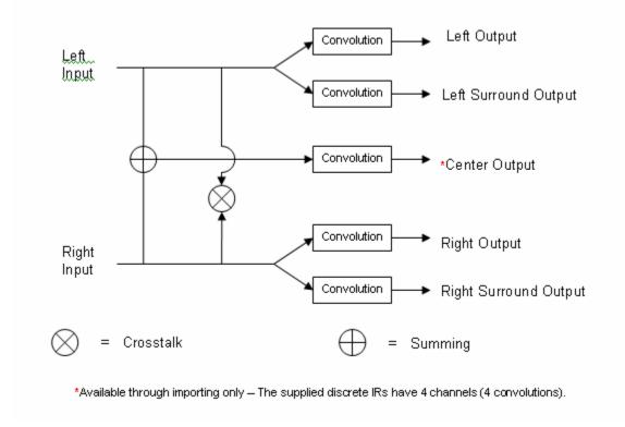
Efficient Stereo to 5 Channel Discrete Surround Processor: 4 or 5 Convolutions
