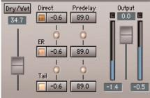
This sets the balance between the "Dry" signal and the convolved signal. 50% Wet setting is the "natural" balance point.
