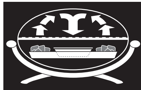
Indirect Method of Cooking One single layer divided into two zones. Add briquettes as needed.
