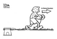
Before actually sinking the cable, run the cable from your unit to the power source or amplifier. Ensure your cable run avoids any obstacles such as sunken sprinkler pipes or piping and electrical cable to your house. Once the cable runs are where you like them, connect your speakers and power source to ensure correct operation <u>before</u> sinking the cable. Disconnect the cable wire at both ends and continue.
