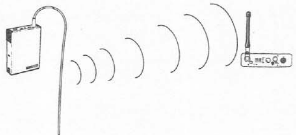
Figure 19 Keeping Site Clear to Antenna
