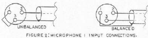
FIGURE 2: MICROPHONE 1 INPUT CONNECTIONS.
