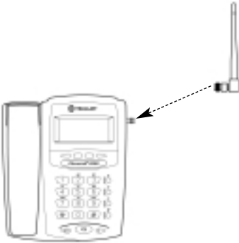
Figure 5 - Attach the antenna.
