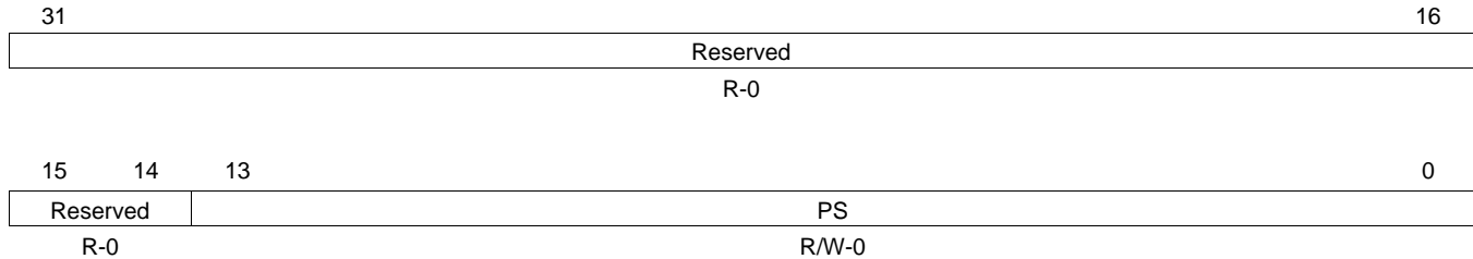
Figure 18. HC Periodic Start Register (HCPERIODICSTART)
