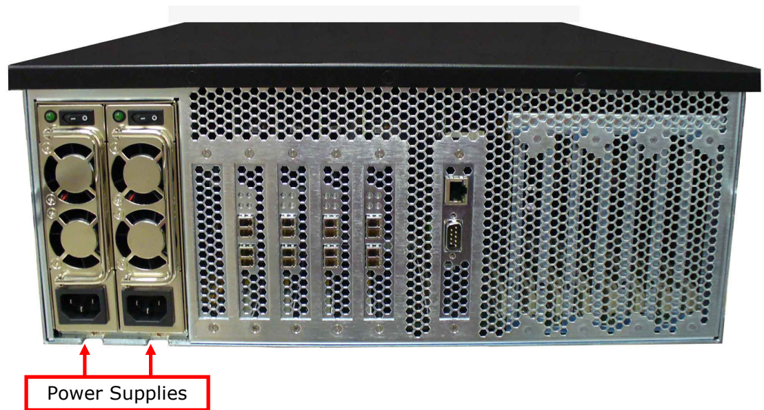
Figure 29 - Back of RamSan-500, Power Supply Location
