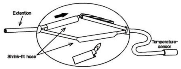
Slide larger tubing (about  $\frac{3}{4}$  ") over the entire completed splice. Heat gently all around until tubing shrinks tight. This connection can then be drawn gently into the pipe work. Only two of the wires are required for the sensor cable; the other two wires are spare wires.
