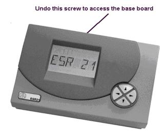
Undo the screw at the top of the housing. The control electronics are mounted on the enclosure cover. The controller enclosure can be screwed to the wall with cable entry grommets pointed downwards. Use the supplied plastic bridges to secure power and sensor cables.
