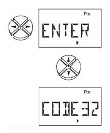
**Par** Using the navigation key  $\Leftrightarrow$  allows you to select the desired parameter while you are in the program mode. Press the selection key  $\clubsuit$  once to select the parameter in the window. Selected parameter **blinks** allowing you to modify it. You can modify the selected parameter while **the middle window blinks** by pressing the  $\Leftrightarrow$  or  $\Rightarrow$  key. The unit accepts the new value by pressing the  $\updownarrow$  key once.
