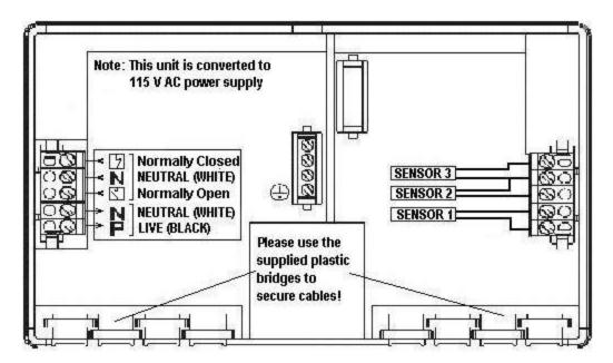
Base of the unit to be mounted at eye-level and wired as shown above
