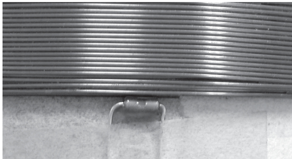
Heat sensor on voice coil
