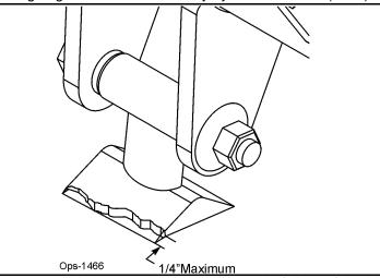
Failure to replace worn or damaged blades may lead to catastrophic failure of the blades and ejection of the broken part with tremendous force which may cause serious bodily injury or death.
