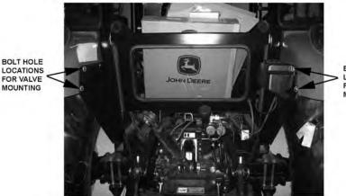
BOLT HOLE LOCATIONS FOR VALVE MOUNTING
