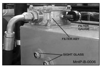
If your reservoir has one sight glass/temperature gage: The reservoir should be filled to the center of the sight glass on the side of the tank. Do not overfill. If the tank has too much oil, the excess may be expelled through the pressurized breather.
