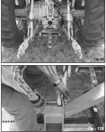
NOTE: Offset Adaptor Hitches are available to position the mower to the left or right. Mowers with Offset Adaptor hitches connect to the 3-Point hitch the same way as the mower A-frame.
