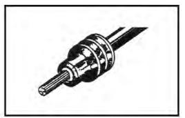
2. Align seal with cable insulation.
