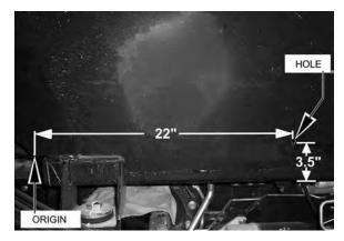
Place as many hoses in the clamp that will fit without compromising pressure. Then secure the (2) HOSE CLAMP (06520013) to the holes drilled with (1 EACH) CAPSCREW,3/8 X 1 NC (21630) and (1 EACH) NYLOCK NUT,3/8 NC (21627). The hoses that don't fit into the clamp are to be secured to the others with zip-ties. For protection of hoses in contact with metal edges, wrap hoses with spit hose sections and fasten with hose clamps or zip ties as needed.
