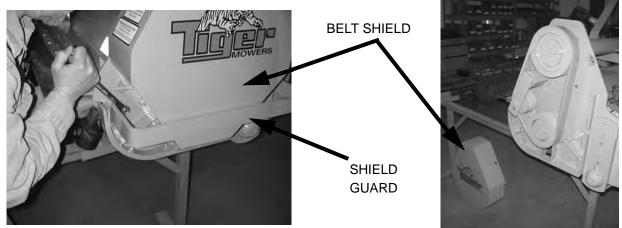
Place a straight edge over both sheaves and measure the belt tension (See TENSIONER MEASUREMENT PROCEDURE). To adjust the Rosta Tensioner, first, loosen the Rosta Stop and Rosta Bolt that secures the Rosta to the flail. Next use the Wrench (P/N 06401023 available) to adjust the tension of the belt. After the tension has been set, secure the Rosta Stop and re-torque the Rosta Bolt to specs.
