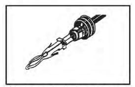
Crimp and visually inspect for a good crimp before installing in connector body.
