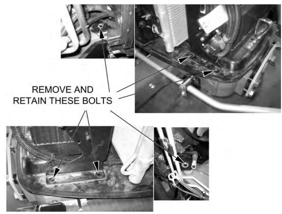
After the bolts have been removed, use a pry bar to raise the battery plate. Once the plate is raised, use an appropriate block to keep the battery plate raised. (ASM-JD-0086)
