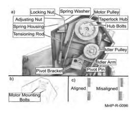
5-Remove the idler pulley from the idler arm and reinstall in the short end of the new idler arm.
